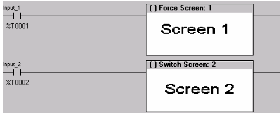
Figure 12.2 – Force and Switch Coils in Ladder Programming
